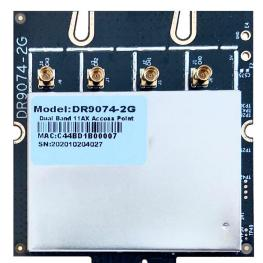
DR9074-2.4G(PN01.1) based on QCN9074 Chipset is an enterprise wireless module integrated with 4x4 MU-MIMO 2.4GHz Single Band Wireless Module designed specifically to provide users with mobile access to high-bandwidth video streaming, voice, and data transmission for office and challenging RF environment in factories, warehouses establishment.
